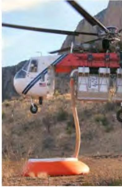
**Figure 29. Rigid tank model shown with helicopter snorkel.**
