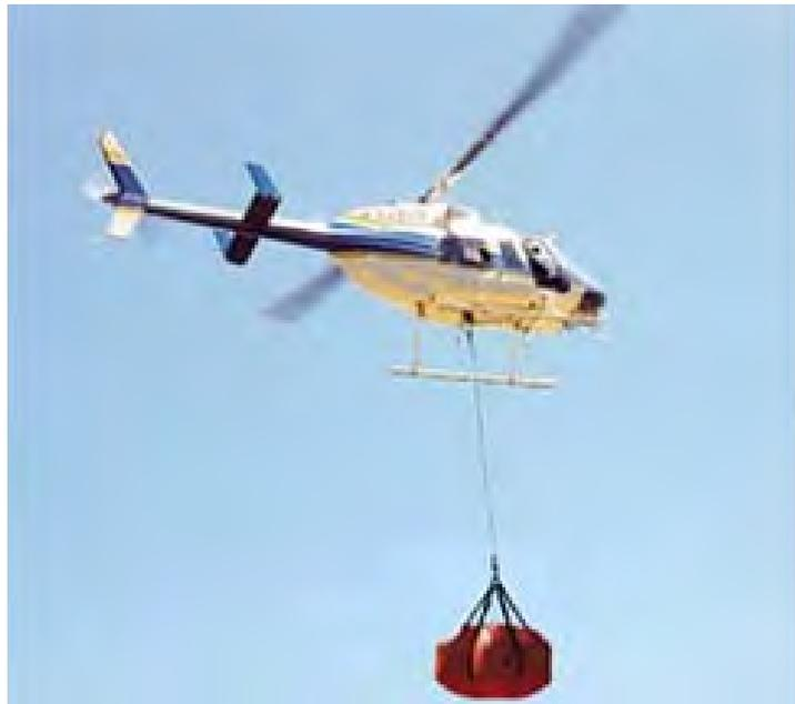
**Figure 30. Soft-sided tank model being airlifted.**
