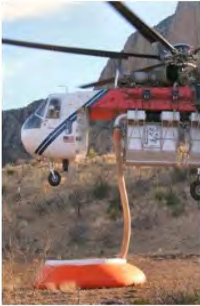
Figure 20. Rigid tank model shown with helicopter snorkel.
