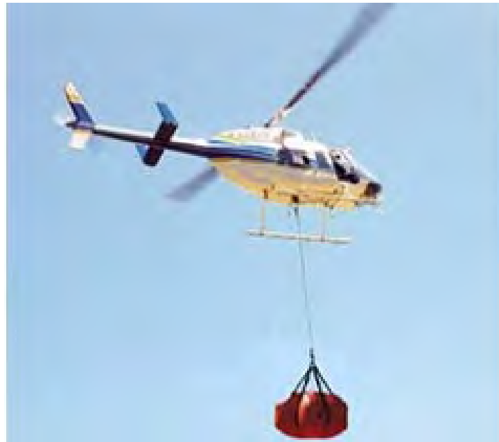
Figure 21. Soft-sided tank model being airlifted.
