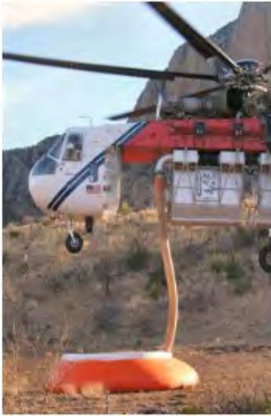
Figure 20. Rigid tank model shown with helicopter snorkel.
