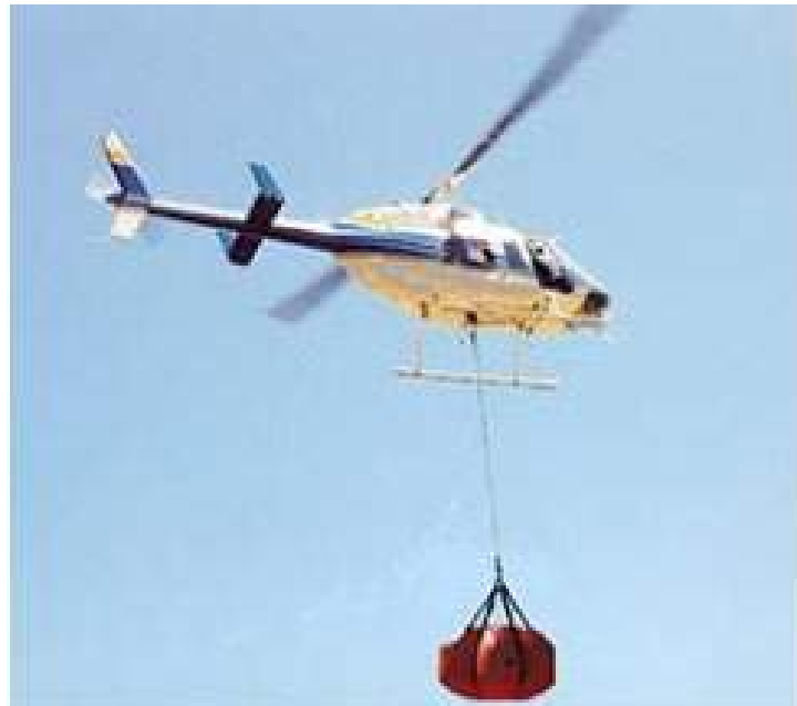
Figure 21. Soft-sided tank model being airlifted.
