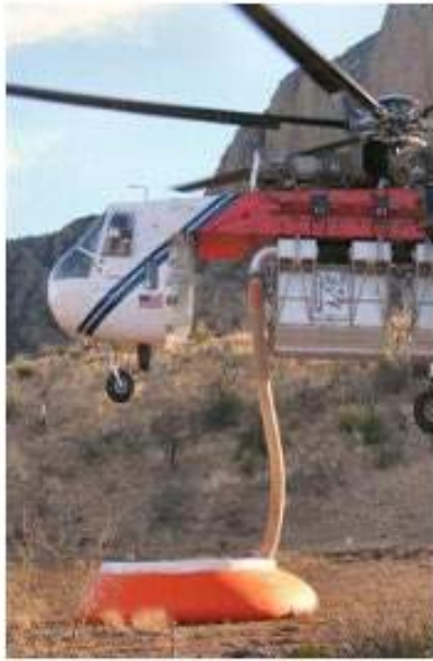
Figure 20. Rigid tank model shown with helicopter snorkel.
