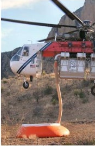
Figure 20. Rigid tank model shown with helicopter snorkel.
