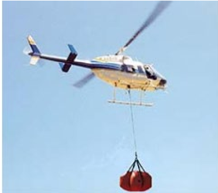
Figure 21. Soft-sided tank model being airlifted.
