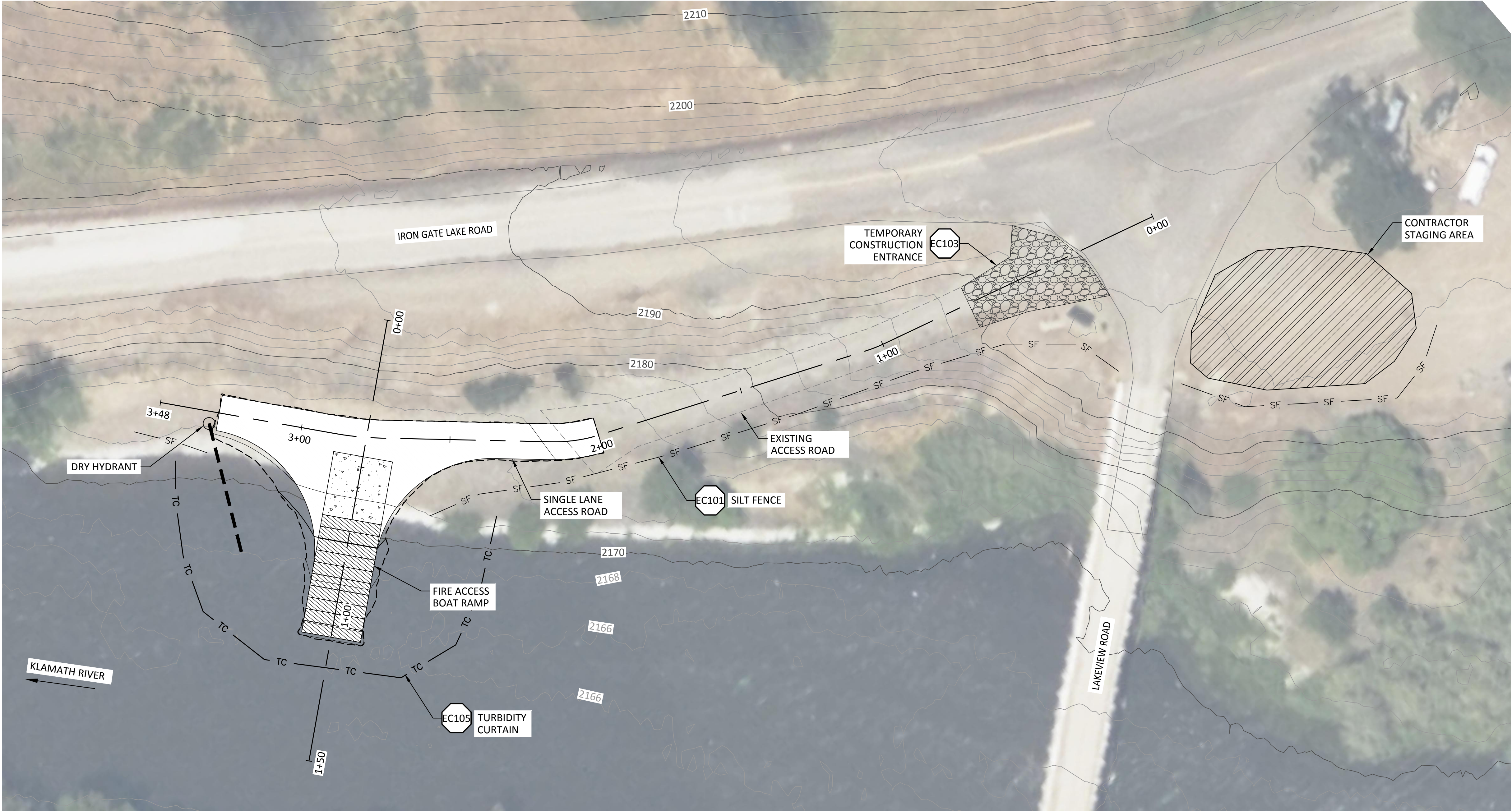
EROSION AND SEDIMENT CONTROL PLAN IRON GATE SCALE: 1" = 20'
