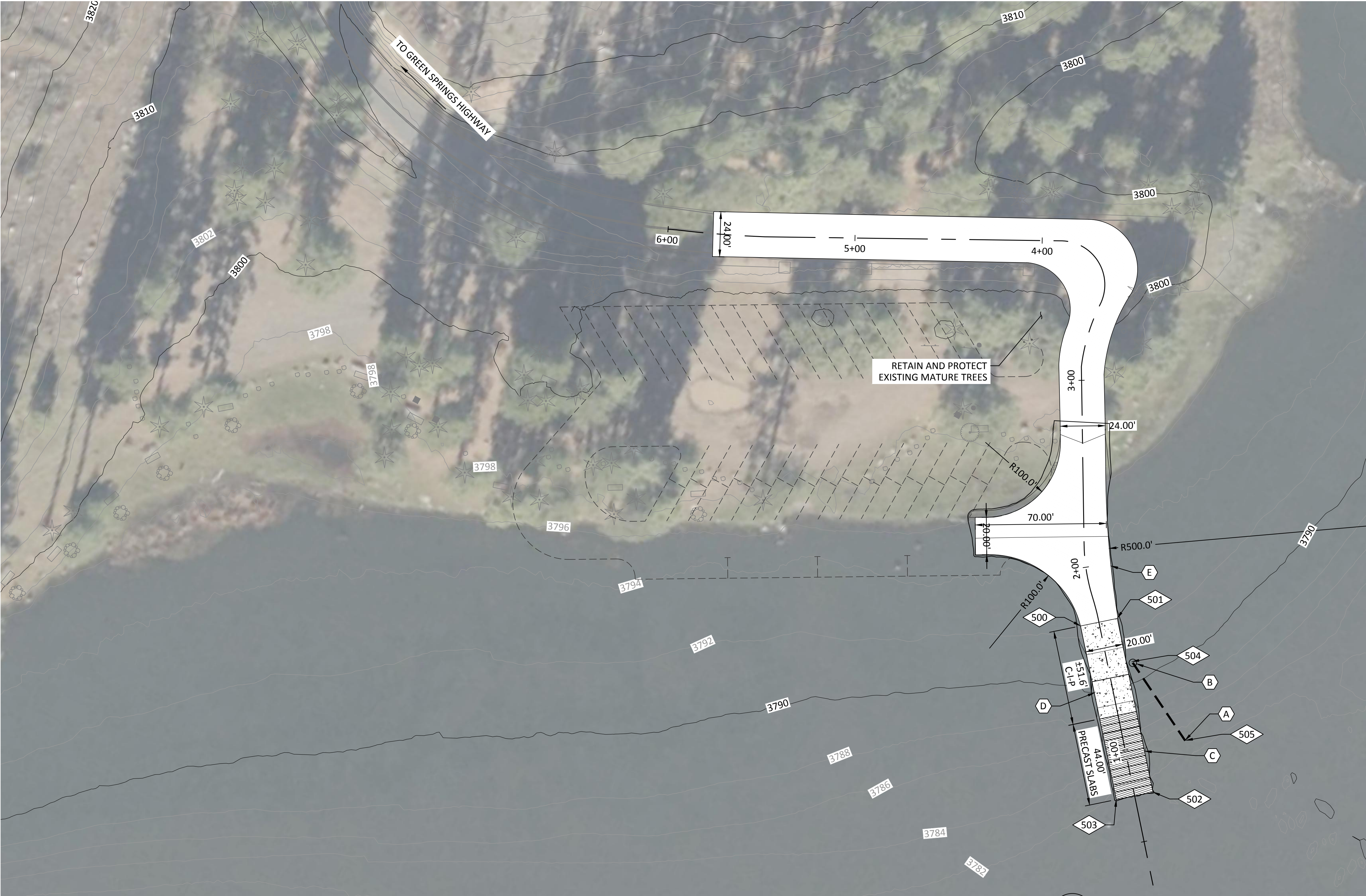
PIONEER PARK WEST FIRE ACCESS BOAT RAMP AND DRY HYDRANT PLAN
