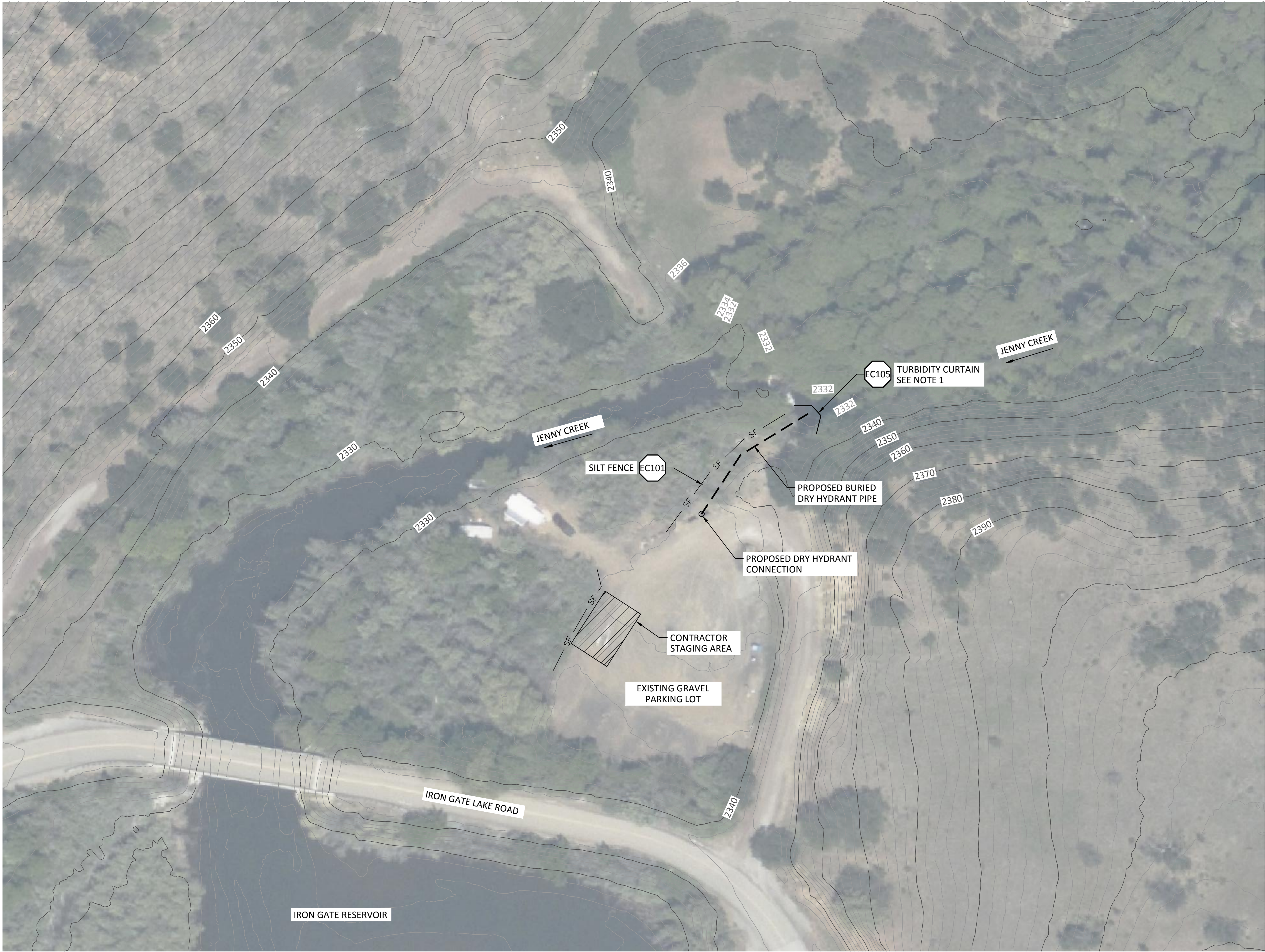
EROSION AND SEDIMENT CONTROL PLAN JENNY CREEK SCALE: 1"= 40'
