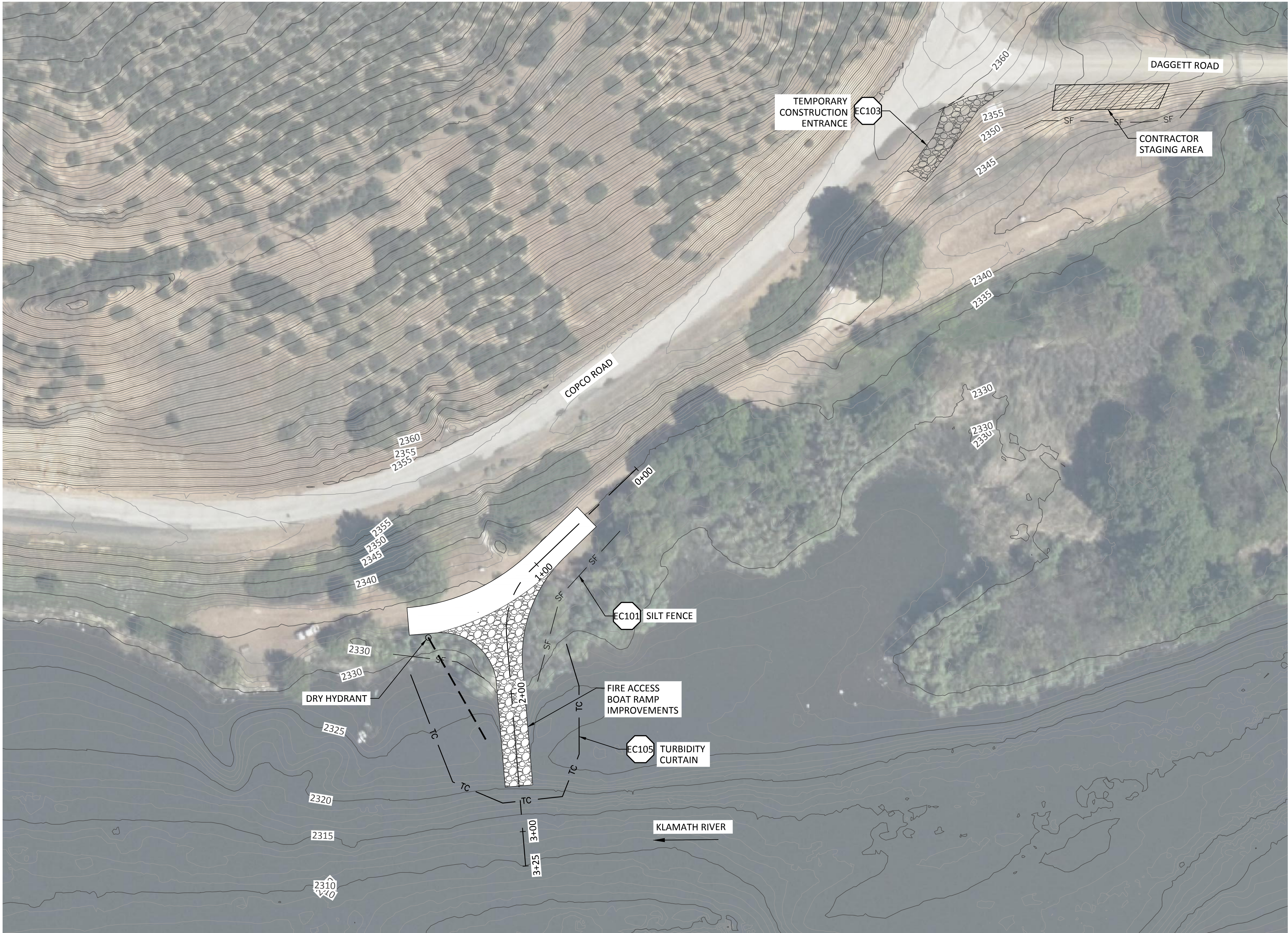
EROSION AND SEDIMENT CONTROL PLAN FALL CREEK CONFLUENCE SCALE: 1"= 40'
