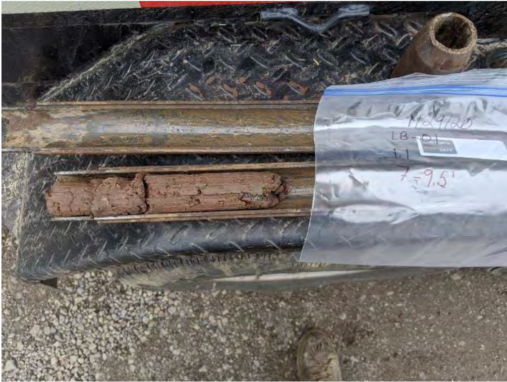
Lakeview Road Bridge Photo 1 – BH-AB01 Sample 1.1 from 7-9.5 ft bgs.
