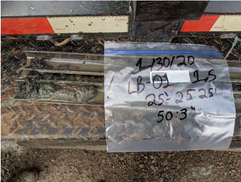
Lakeview Road Bridge Photo 5 – BH-AB01 Sample 1.5 from 25-25.25 ft bgs.
