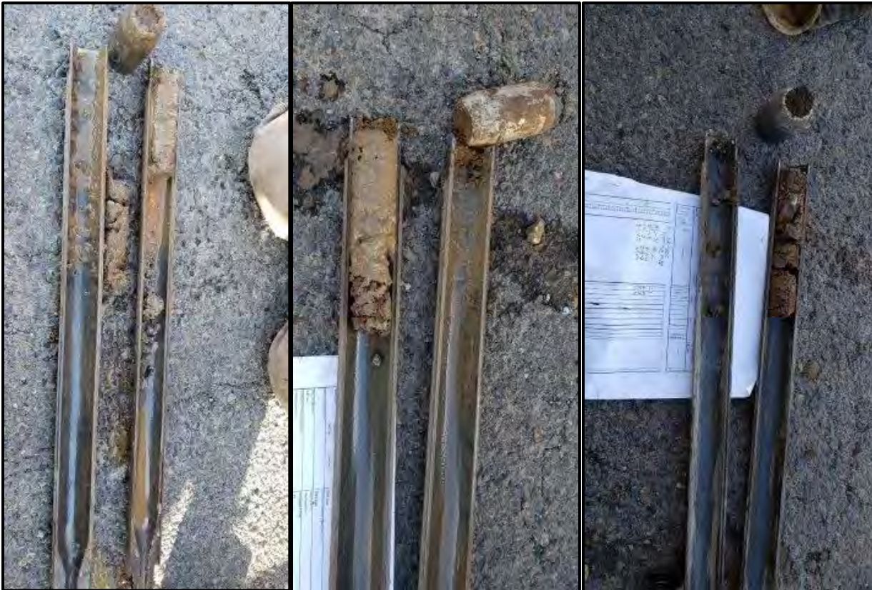
Photograph 3/4/5. SPT samples taken at 0-1.5' bgs -Left, 1.5-3' bgs -Middle, & 3-4.5' bgs -Right (CR-RC-002).
