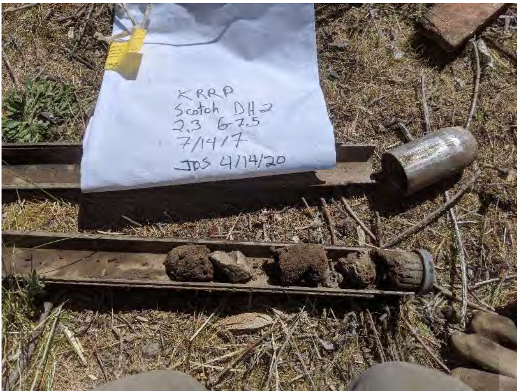
Scotch Creek Culvert Photo 4 – BH-SC02 Sample 2.3 from 6-7.5 ft bgs.
