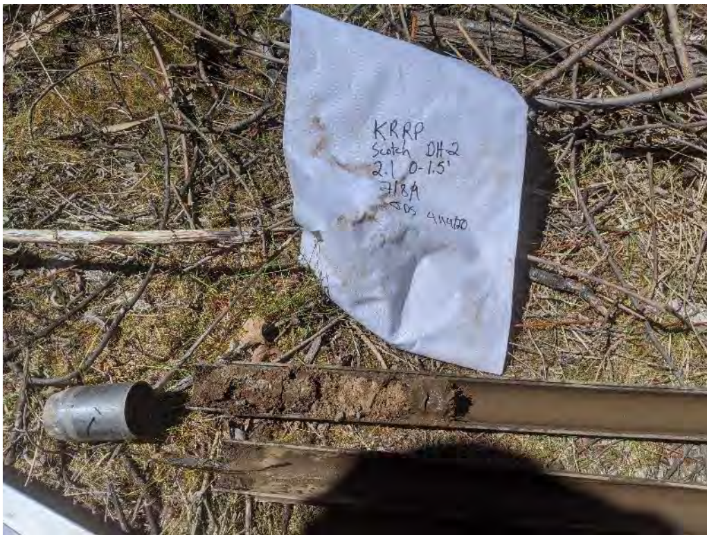
Scotch Creek Culvert Photo 2 – BH-SC02 Sample 2.1 from 0-1.5 ft bgs. #
