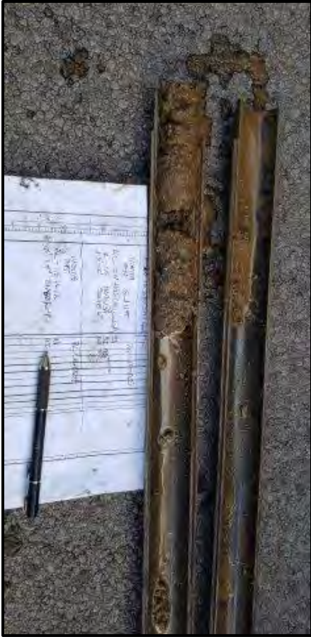
Photograph 13. SPT sample taken at 0-0.8' bgs (CR-RC-004).
