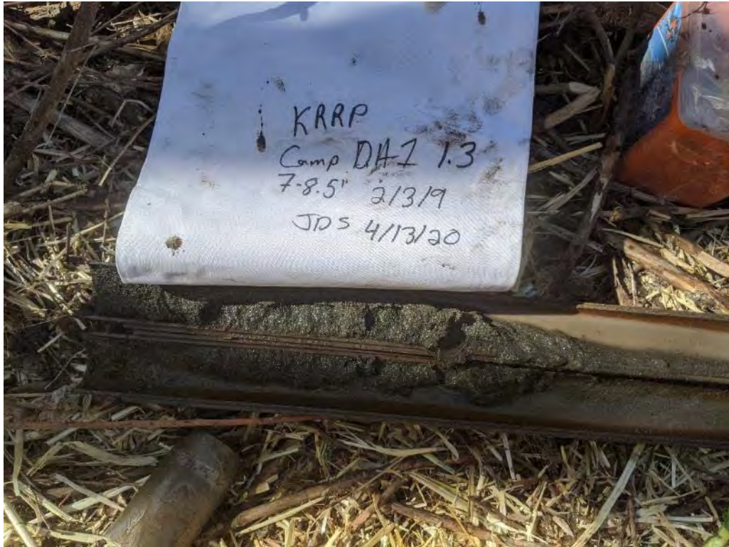
Camp Creek Culvert Photo 1 – BH-CC01 Sample 1.3 from 7-8.5 ft bgs. #
