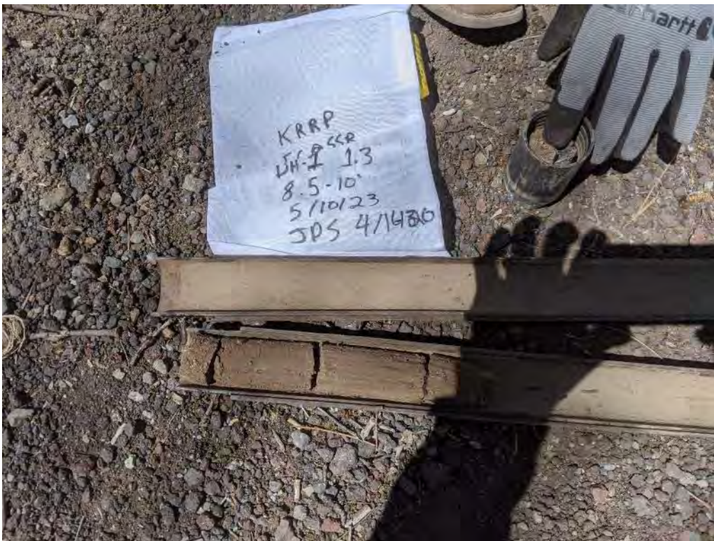
Fall Creek at Substation Road Photo 2 – BH-DG02 Sample 1.3 from 8.5-10 ft bgs.
