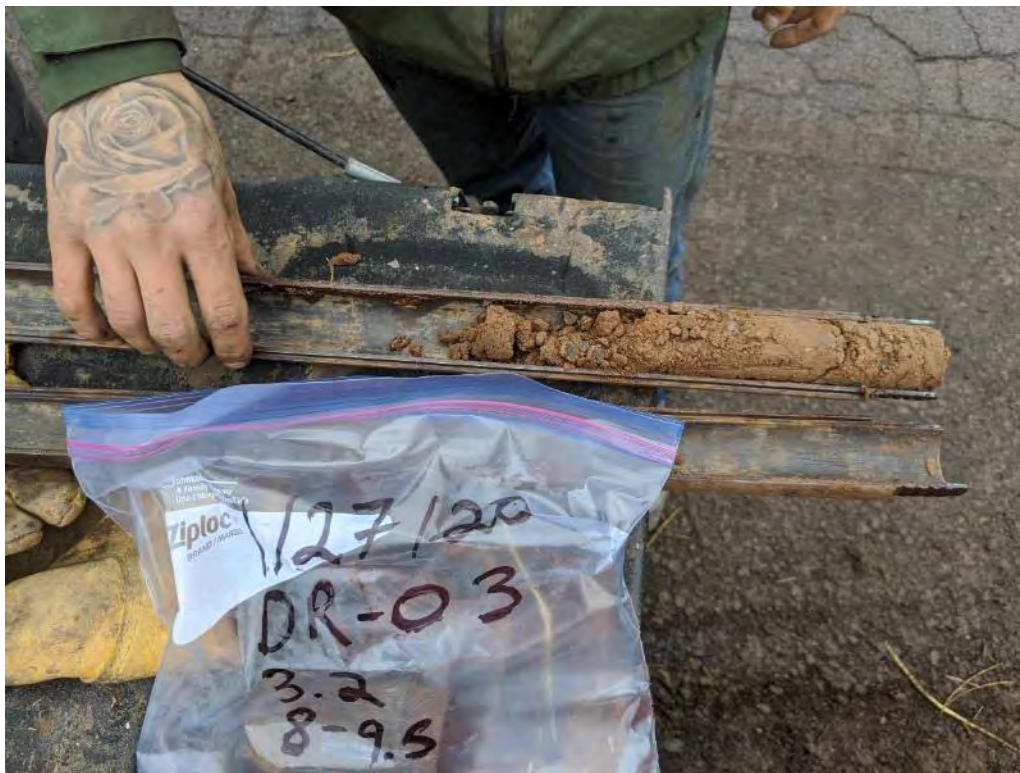
Copco Road at Dry Creek Bridge Photo 2 – BH-DR03 Sample 3.2 from 8-9.5 ft bgs.
