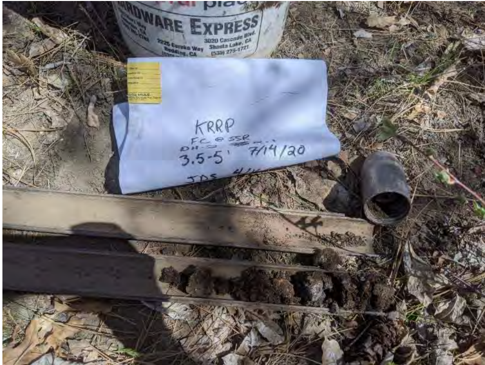
# Fall Creek at Substation Road Photo 3 – BH-DG01 Sample 2.1 from 3.5-5 ft bgs.
