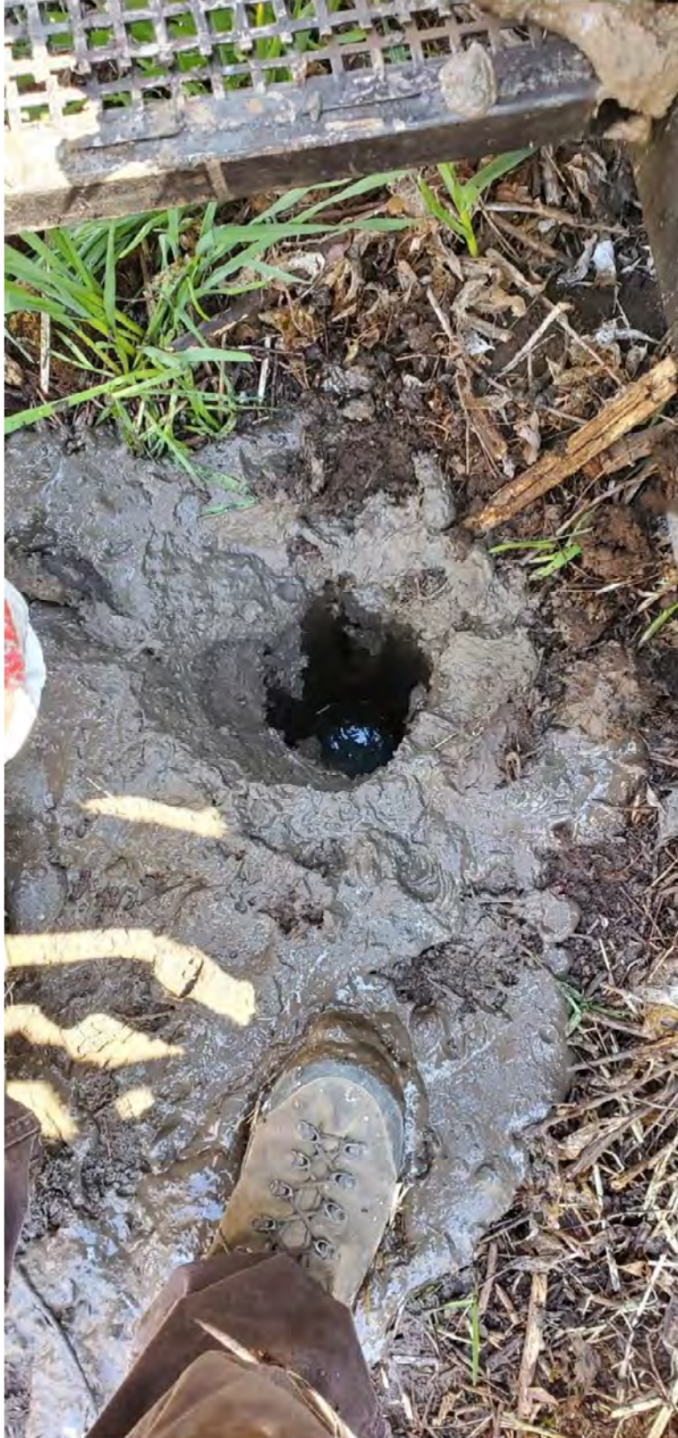
Camp Creek Culvert Photo 3 – BH-CC01 immediately after drilling completion, ground water present in borehole.
