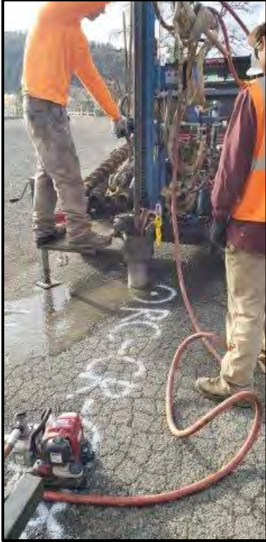
Photograph 17. Looking at asphalt coring at Road Core RC-CR-006 (STA 430+68.0).
