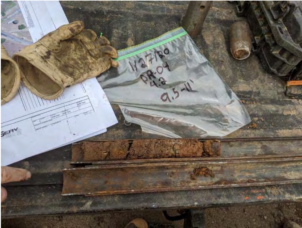
# Copco Road at Dry Creek Bridge Photo 3 – BH-DR04 Sample 4.2 from 9.5-11 ft bgs.
