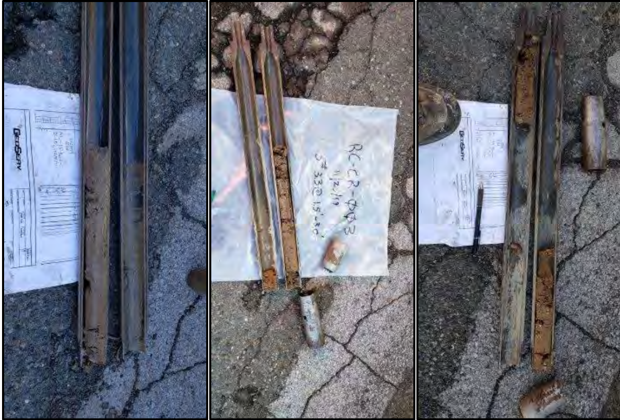
Photographs 8/9/10. SPT samples taken at 0-1.5' bgs- Left , 1.5'-3.0' bgs- Middle , & 3.0-4.5' bgs- Right (CR-RC-003).
