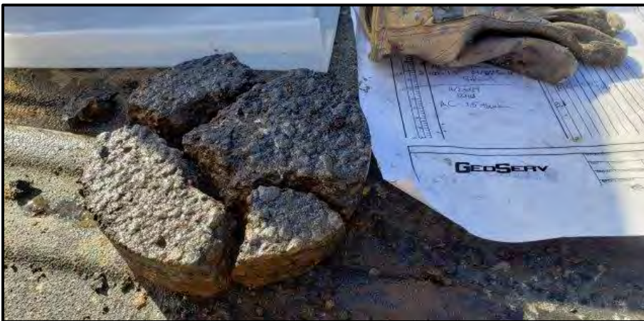
Photograph 7. Asphalt core sample at Road Core RC-CR-003 ( STA 220+57.0 ).
