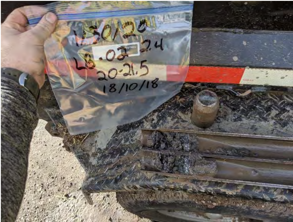
Lakeview Road Bridge Photo 7 – BH-AB2 Sample 2.4 from 20-21.5 ft bgs.
