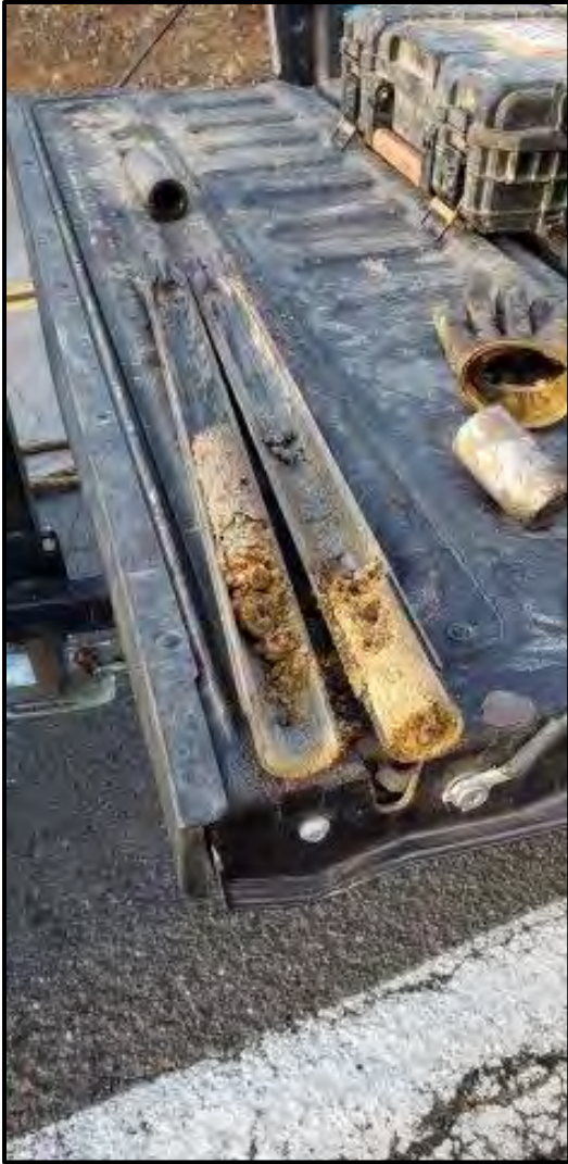
Photographs 1. Road Core RC-CR-001 (STA 180+60.0) SPT sample taken from 0-1.5' bgs.
