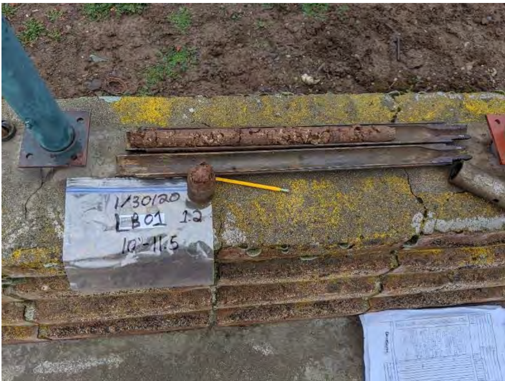
Lakeview Road Bridge Photo 2 – BH-AB01 Sample 1.2 from 10-11.5 ft bgs.
