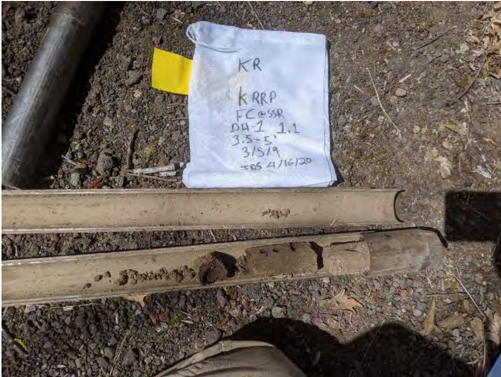
Fall Creek at Substation Road Photo 1 – BH-DG02 Sample 1.1 from 3.5-5 ft bgs. #
