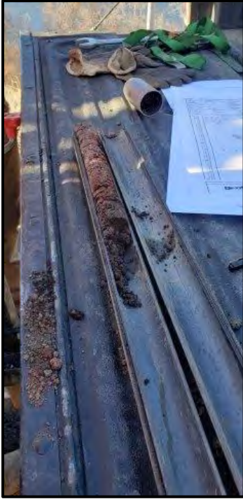
Photograph 29. Looking at SPT sample taken from 0.5-2.5' bgs (RC-CR-09A).
