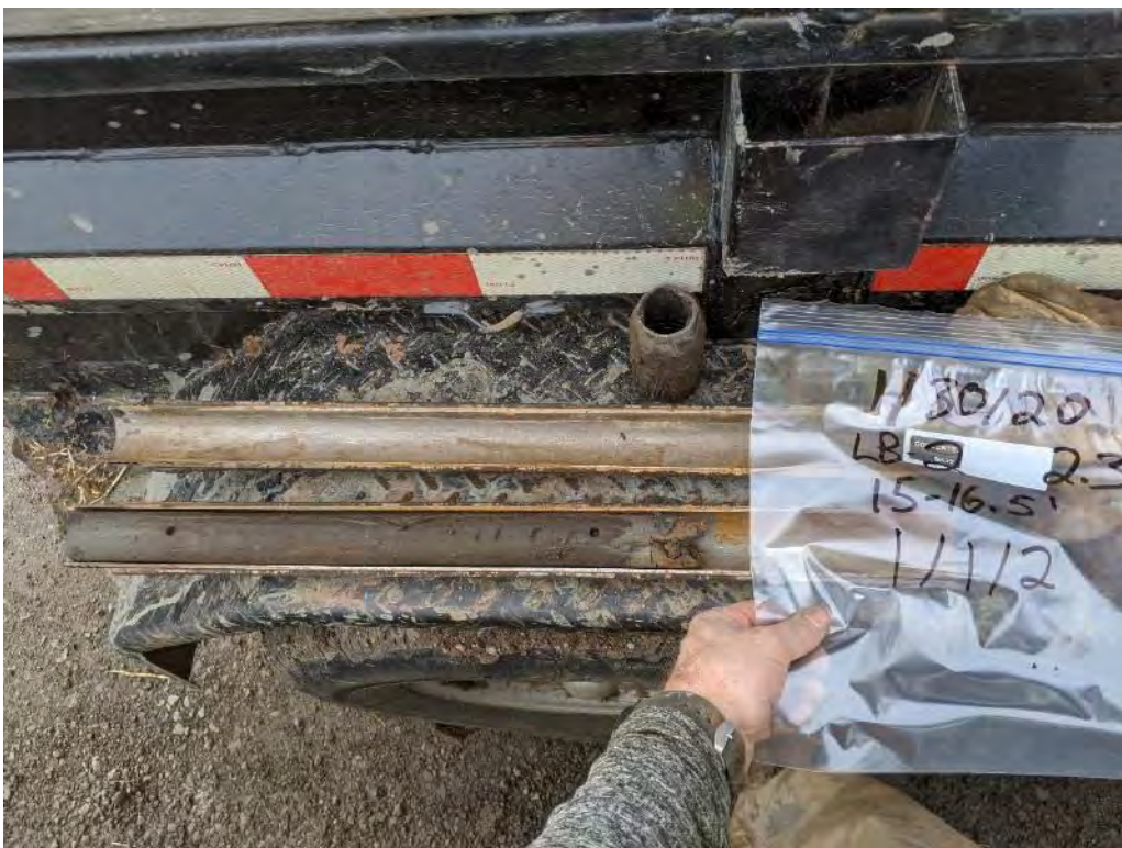
Lakeview Road Bridge Photo 6 – BH-AB02 Sample 2.3 from 15-16.5 ft bgs.
