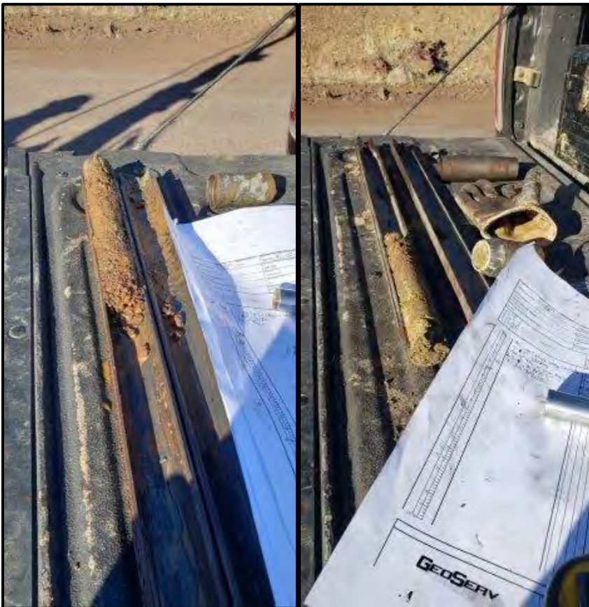
Photographs 22 & 23. SPT samples taken at 0-1.5' bgs-Left, & 2.5-4.0' bgs-Right (CR-RC-008)
