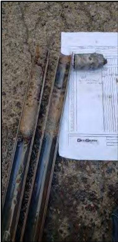
Photograph 18. SPT sample taken at 0-1.5' bgs (CR-RC-006)
