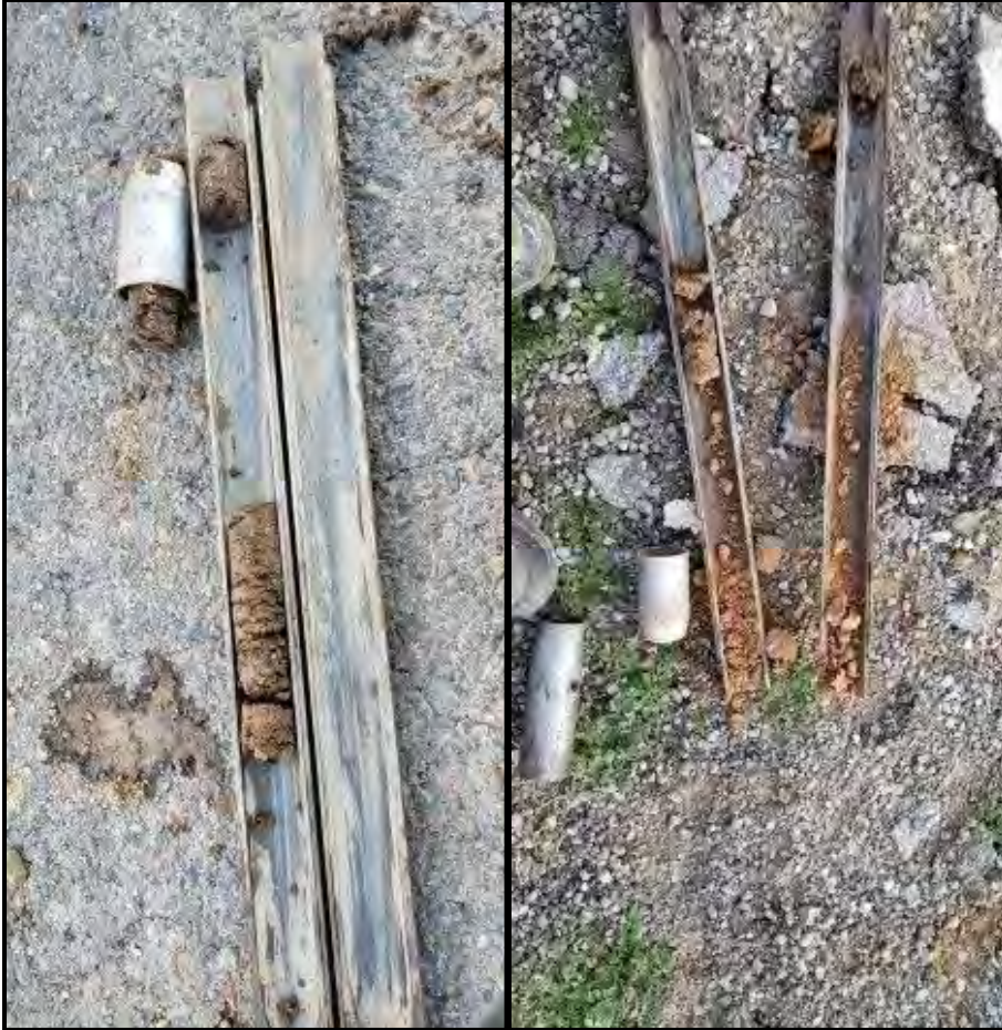
Photograph 6 & 7. SPT sample taken at 4.5-6.0' bgs- Left , & 6.5-6.584' bgs- Right (CR-RC-002).
