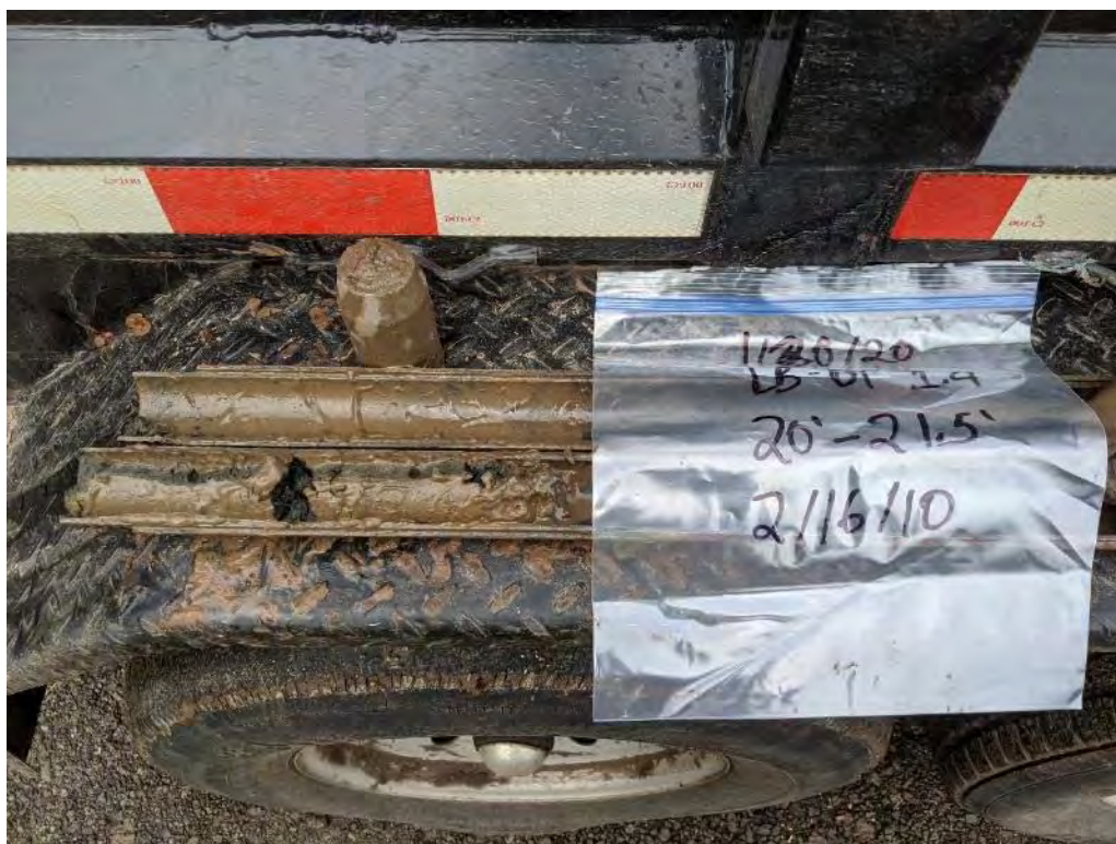
Lakeview Road Bridge Photo 4 – BH-AB01 Sample 1.4 from 20-21.5 ft bgs.
