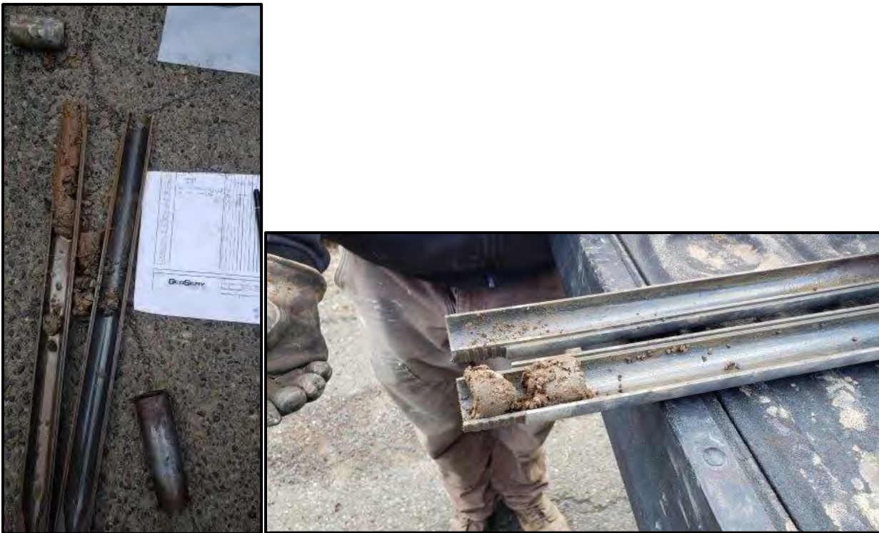
Photograph 15 & 16. SPT samples taken at 0-1.5' bgs -Left, & 1.5-1.958' bgs-Right (CR-RC-005)
