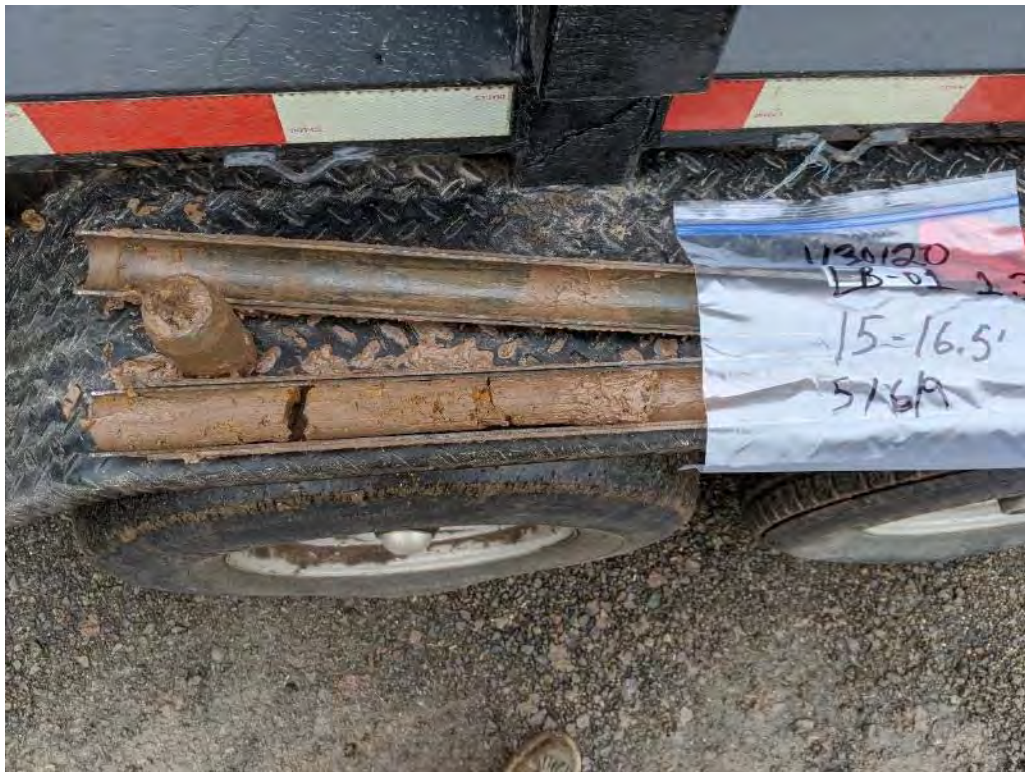
Lakeview Road Bridge Photo 3 – BH-AB01 Sample 1.3 from 15-16.5 ft bgs.
