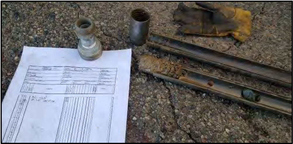
Photograph 20. SPT sample taken at 0-0.8' bgs (CR-RC-007)
