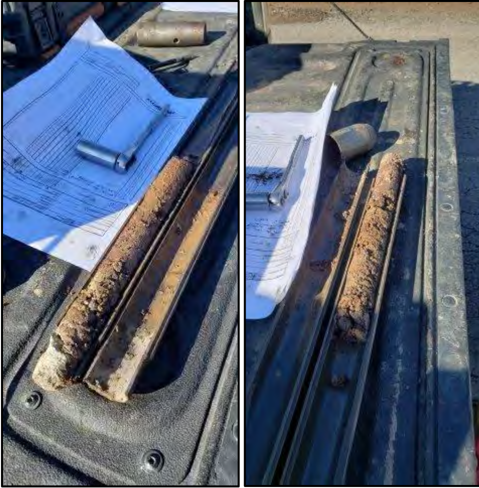
Photograph 26 & 27. SPT samples taken at 0-1.5' bgs -Left, & 1.5-3.0' bgs -Right (CR-RC-009)
