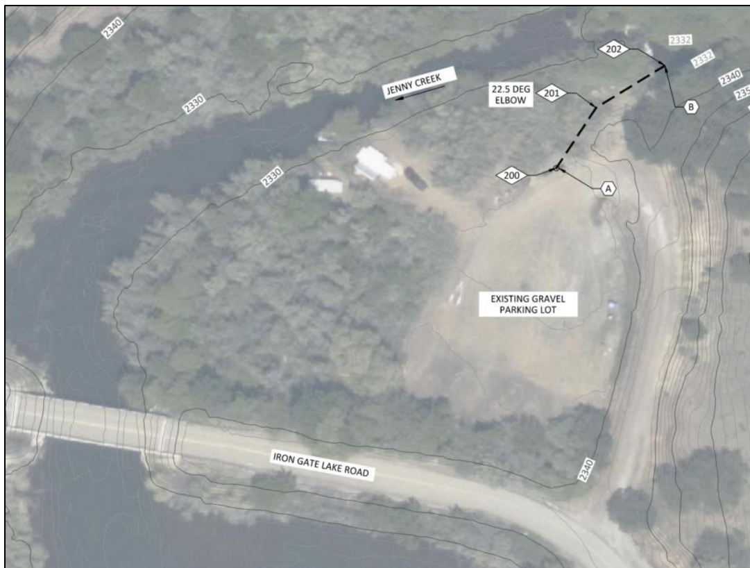
Figure 2-2. Jenny Creek Dry Hydrant
