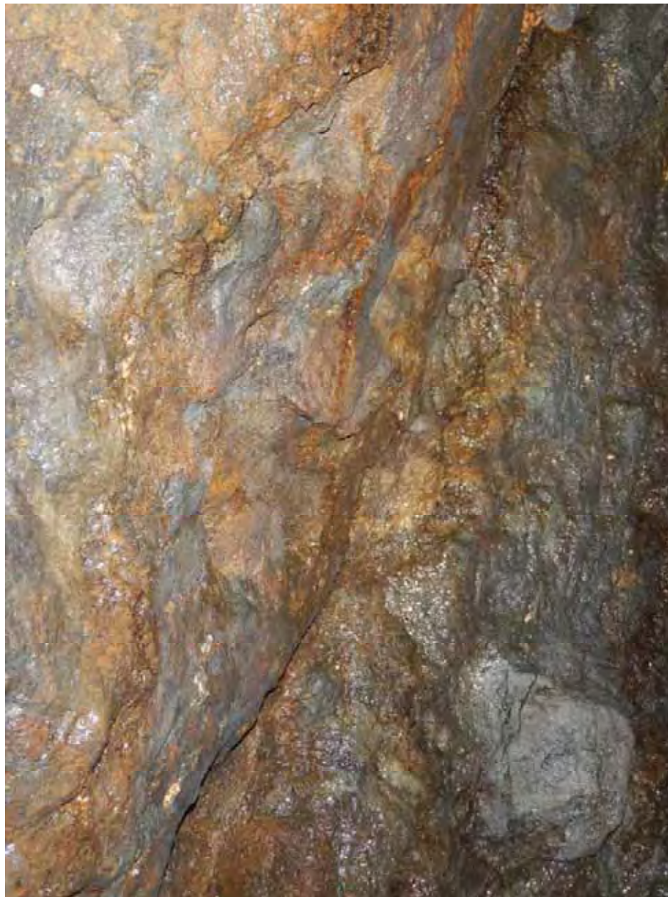
STA. 124.7 to 145.0 ft - Highly persistent Set 1 Joint, 1-inch wide with soil infill comprising weak to medium strong gravel size rock fragments with trace to some sand and trace clay
