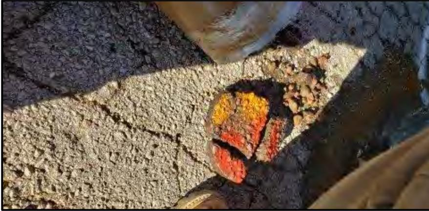
**Photograph 21.** Asphalt core sample at Road Core RC-CR-008. (507+44.0)
