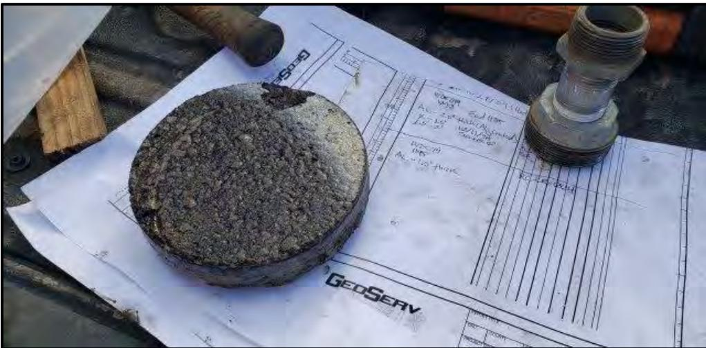
**Photograph 12.** Asphalt core sample at Road Core RC-CR-004.
