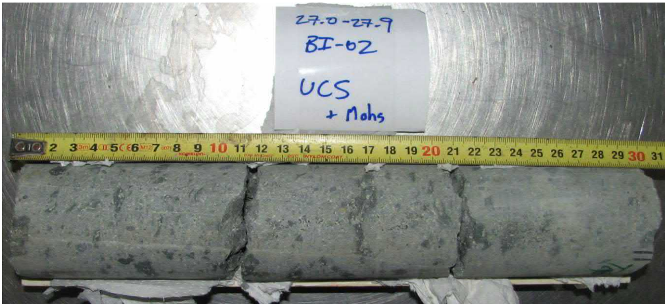
Picture of the sample upon arrival at Tonon USA Laboratory: no core piece allowed preparation of a specimen with a height-to-diameter ratio between 2 and 2.5.
