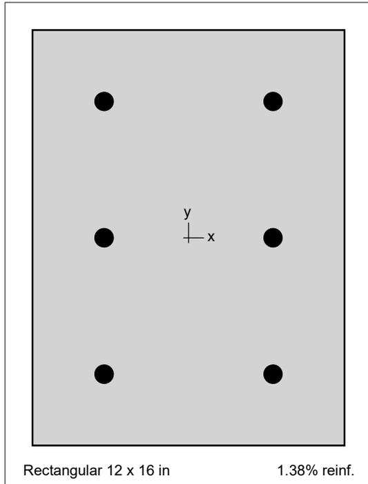
Figure 1: Column section
