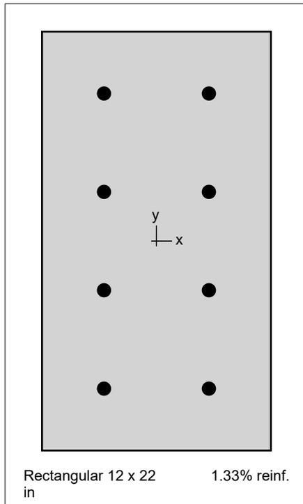
Figure 1: Column section
