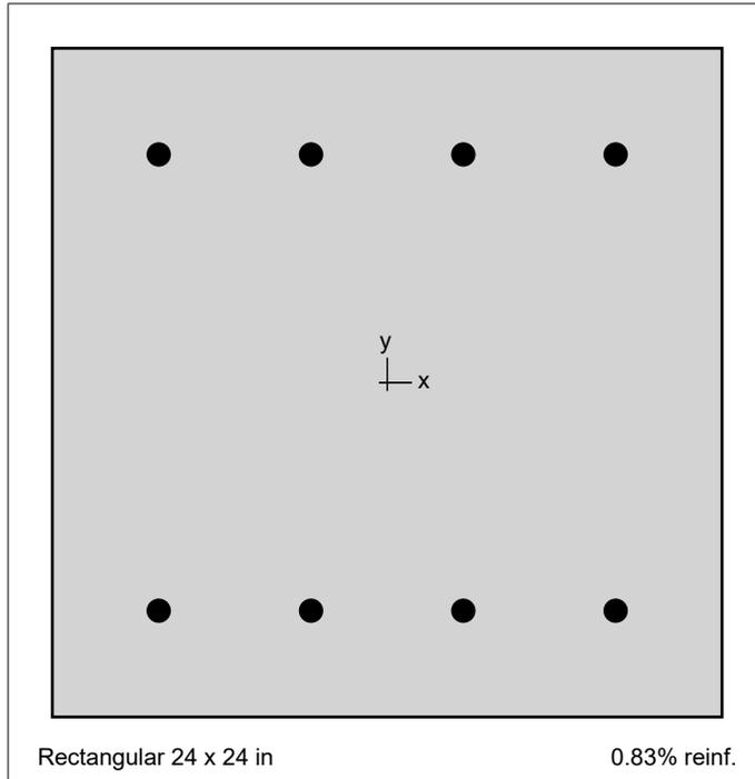
Figure 1: Column section
