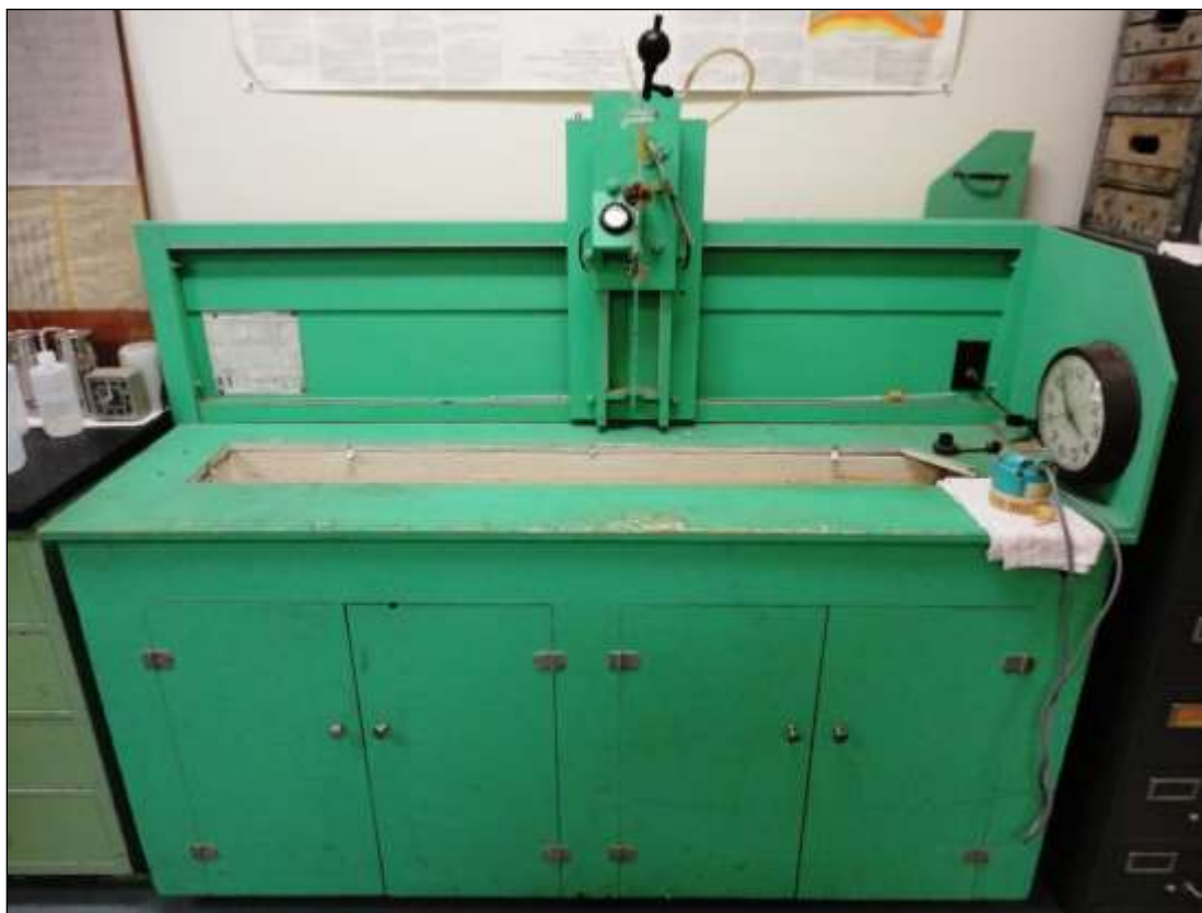
Figure 5: Pipet Bath used for performing particle size analysis via the pipet method.
