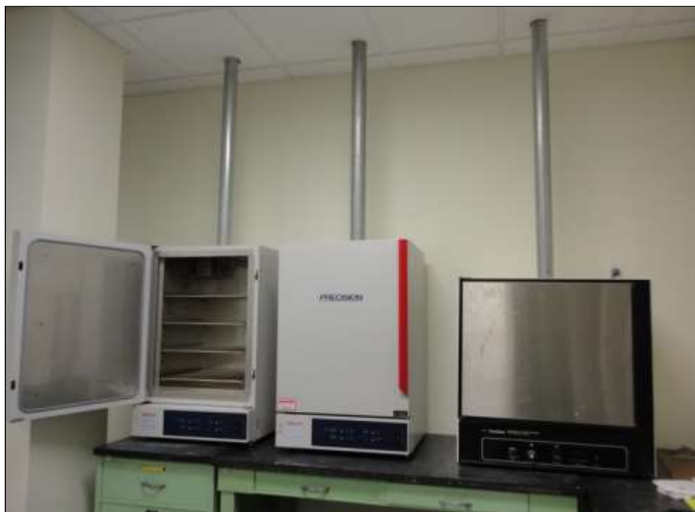
Figure 2: Three mechanical convection ovens used to dry sediment, crucibles, dishes, sample containers and other laboratory items.
