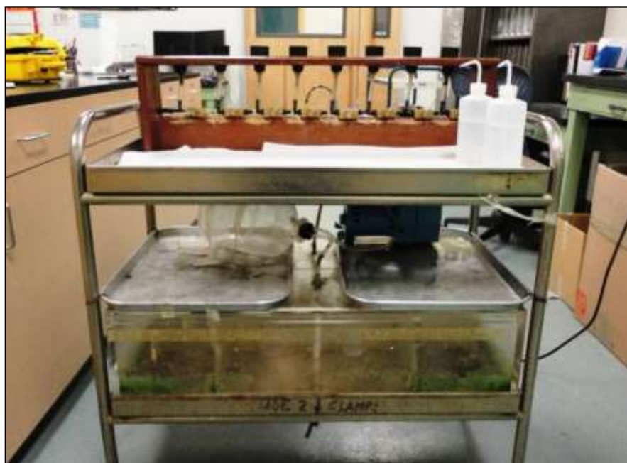
Figure 4: Filtering cart used for sediment analysis. The cart is equipped with a valve operated crucible holding rack, vacuum system and storage tank.
