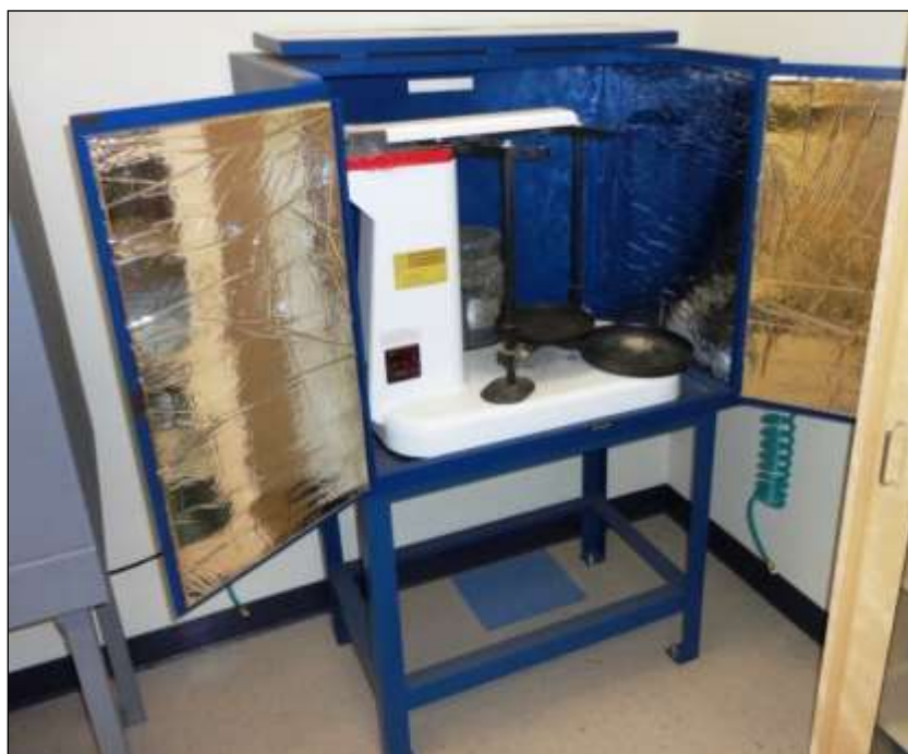
Figure 7: Ro-Tap sieve shaker with sound enclosure and test stand to contain dust and sound.
