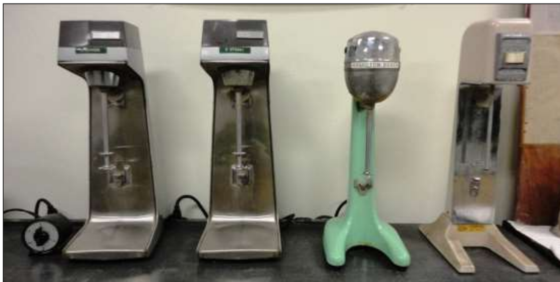
Figure 6: Sediment sample mixers used for mixing and dispersing sediment-water mixture.
