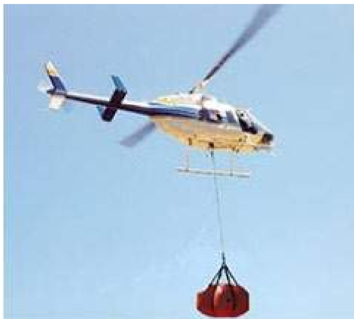
Figure 21. Soft-sided tank model being airlifted.
