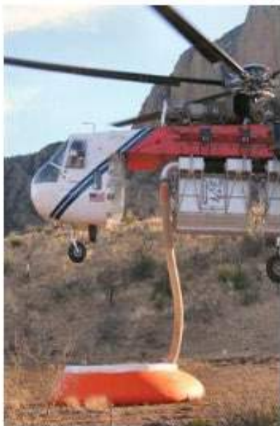
Figure 20. Rigid tank model shown with helicopter snorkel.
