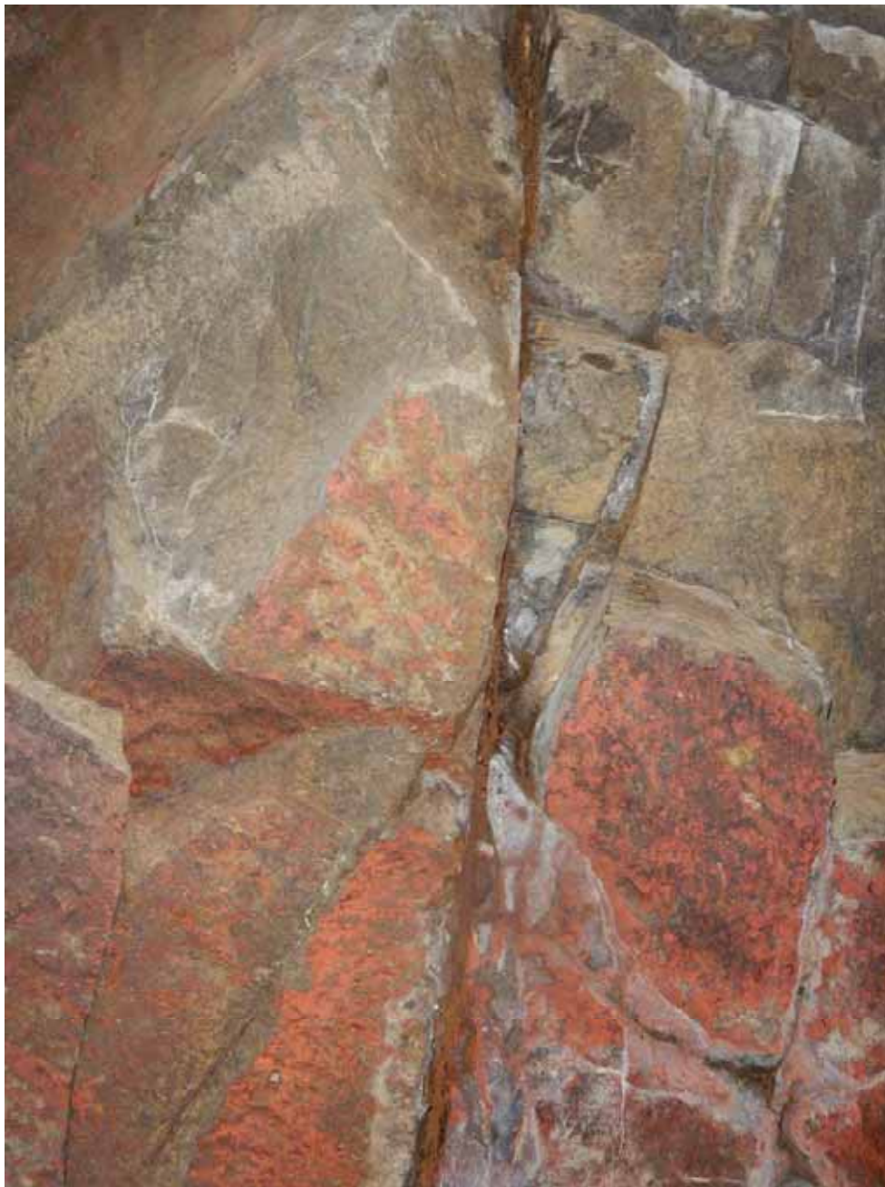
STA. 253.6 ft – Very Steep Set 2 Joint with 1/16 to 1/4-inch of sandy clay infill
