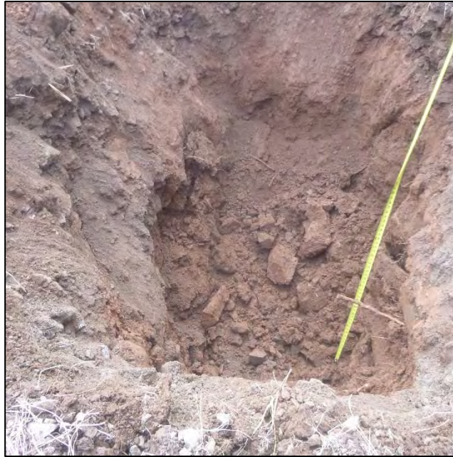
PHOTO 135 – TP-JCB- E pit excavated to depth 6.0 ft
