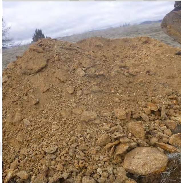
PHOTO 80 – TP-IG-D spoils from excavated depth 4.0 ft to 7.0 ft
