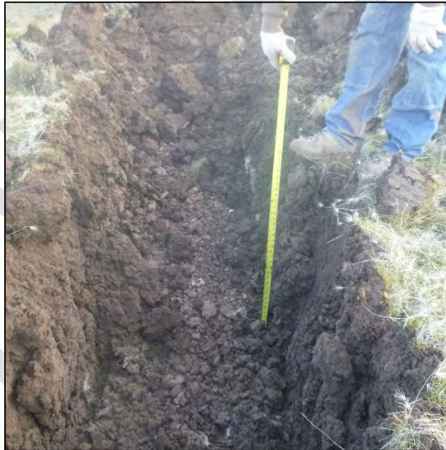
PHOTO 54 – TP-IG-A pit excavated to depth 3.1 ft
