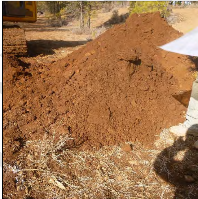
PHOTO 128 – TP-JCB-D spoils from depth 7.7 ft
