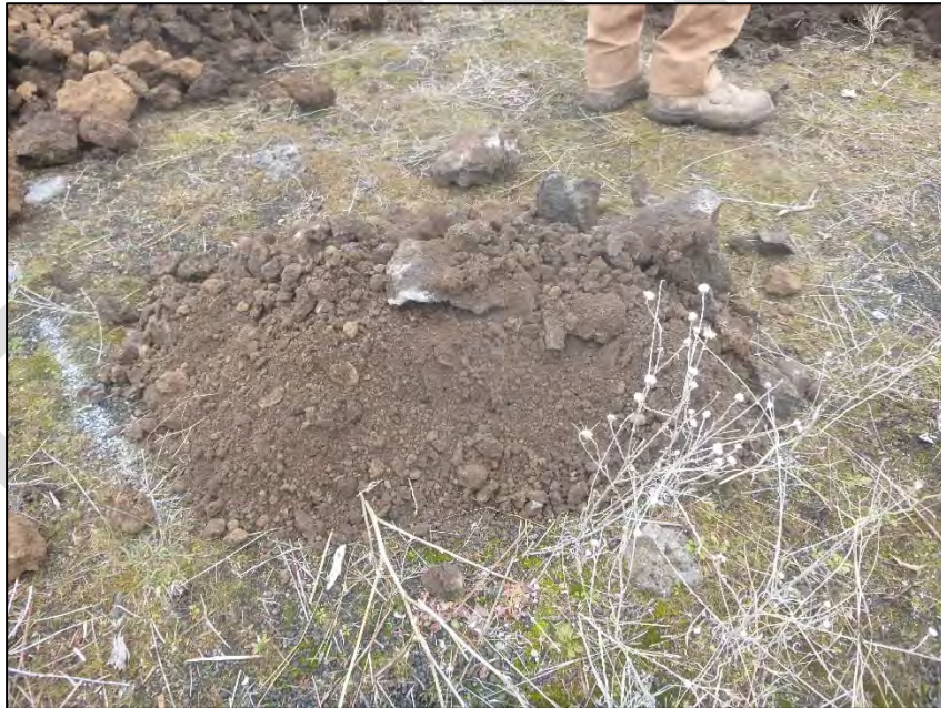
PHOTO 20 – TP-CO1-C spoils from excavation to depth 5.3 ft
