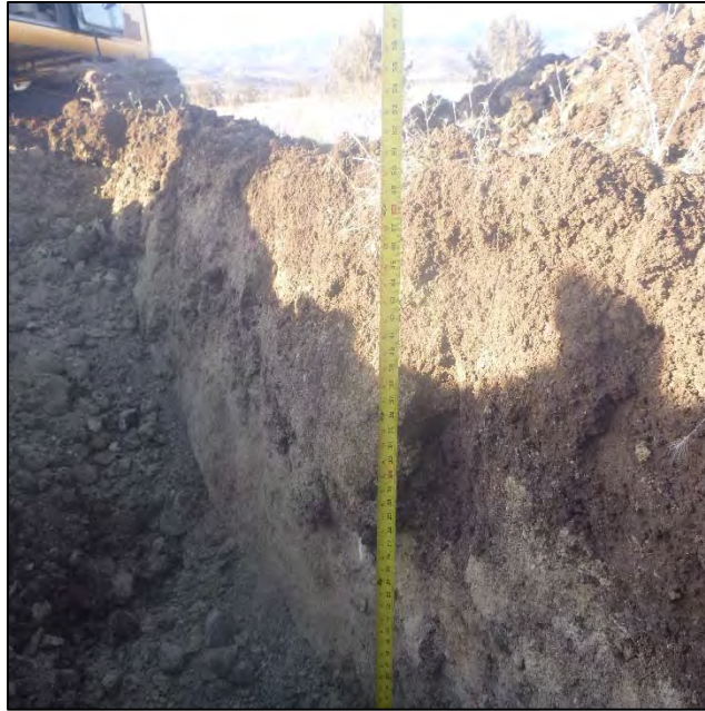
PHOTO 71 – TP-IG-C pit excavated to depth 4.0 ft
