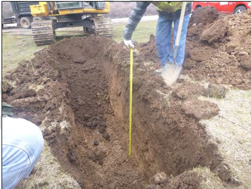
PHOTO 10 – TP-CO1-B excavated to depth 4.0 ft
