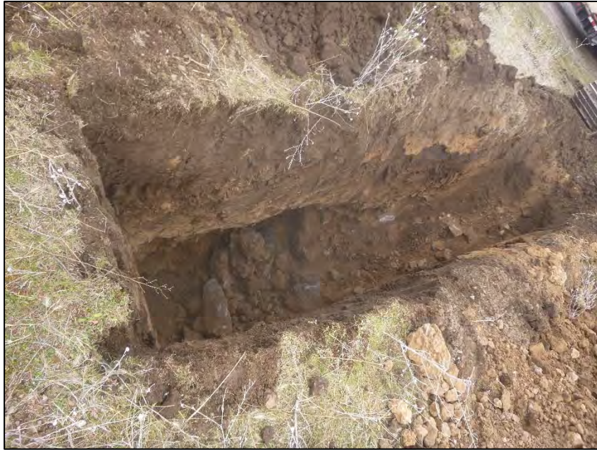
PHOTO 29 – TP-CO1-D pit excavated to final depth approximately 8.8 ft
