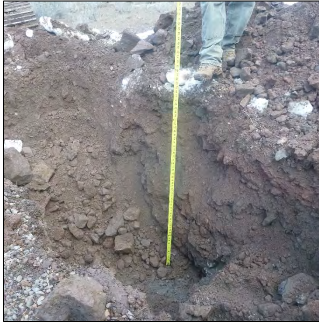
PHOTO 151 – TP-JCB-G pit excavated to depth 4.9 ft
