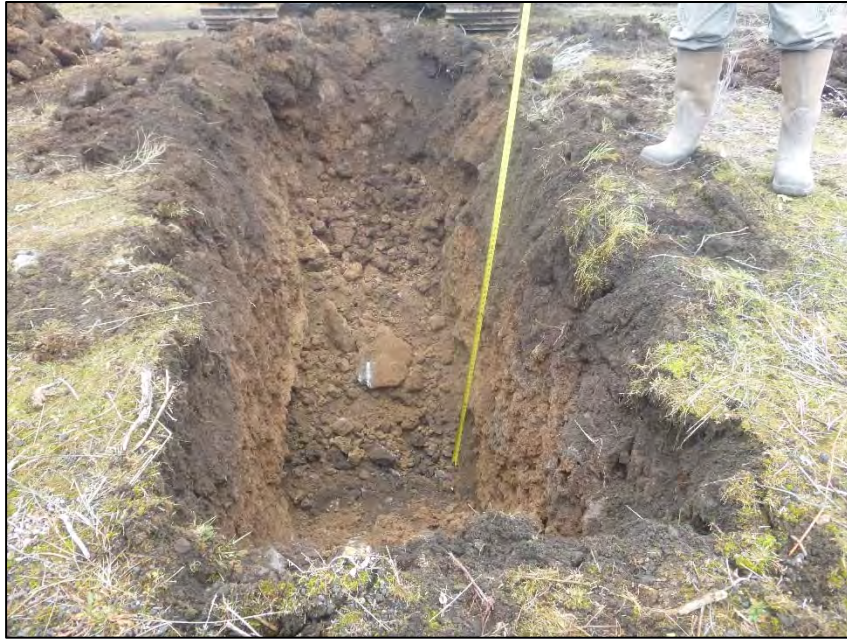
PHOTO 19 – TP-CO1-C pit excavated to depth 5.3 ft
