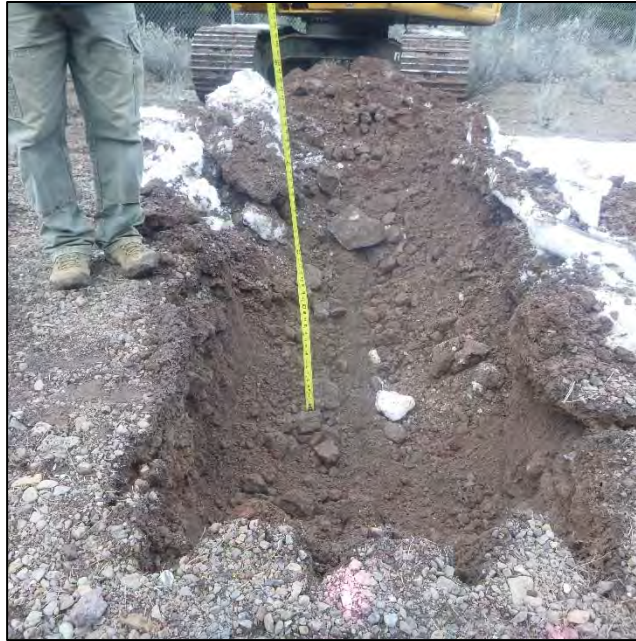
PHOTO 149 – TP-JCB-G pit excavated to depth 1.8 ft
