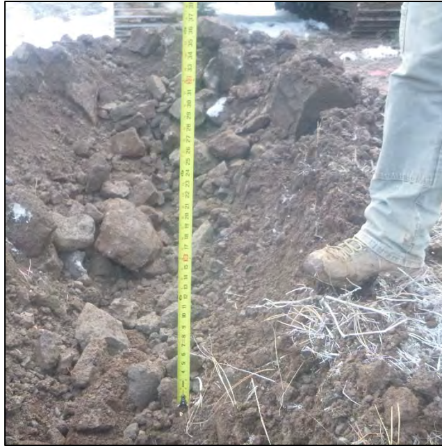
PHOTO 133 – TP-JCB-E pit excavated to depth 1.2 ft
