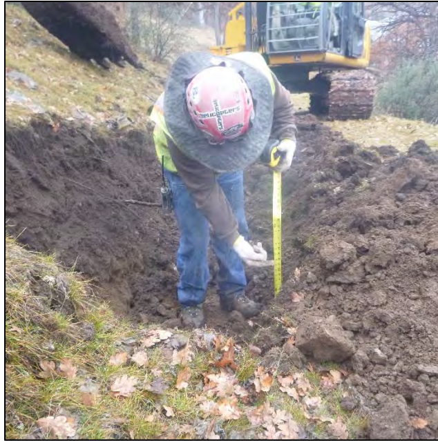
PHOTO 45 – TP-CO2-B pit excavated to depth 1.4 ft
