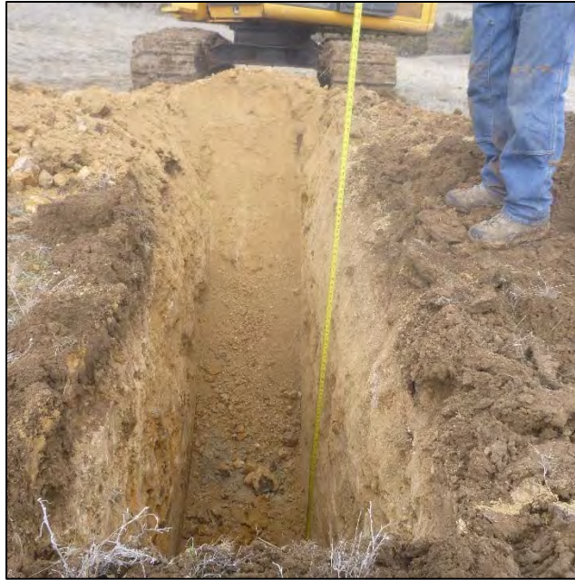
PHOTO 79 – TP-IG-D pit excavated to depth 7.0 ft
