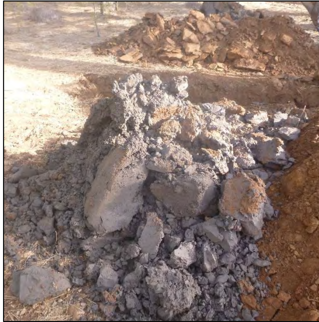
PHOTO 109 – TP-JCB-B spoils from depth 6.6 ft
