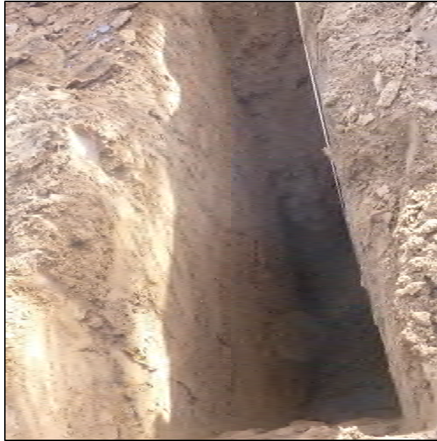
PHOTO 99 – TP-JCB-A pit excavated to depth 12.2 ft
