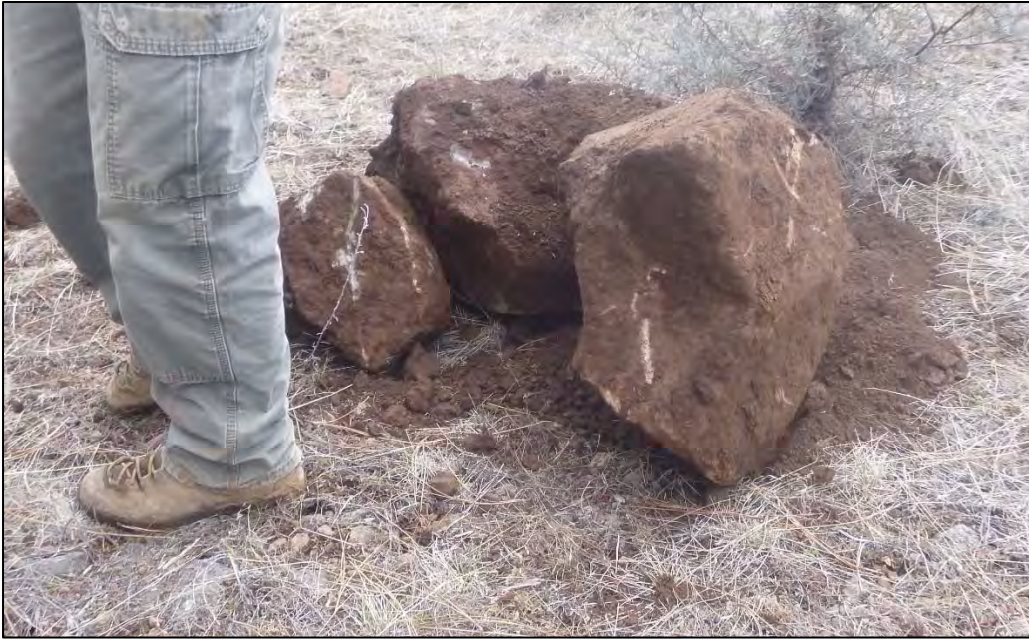
PHOTO 141 – TP-JCB-F boulders uncovered from depth 2.3 to 6.4 ft
