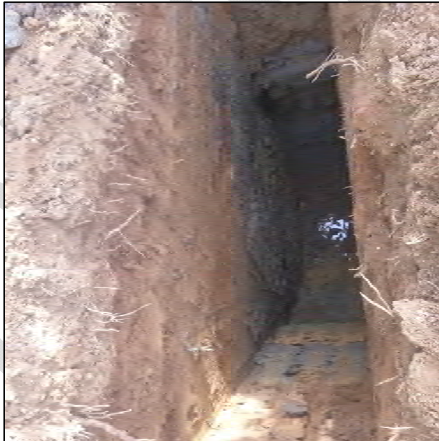
PHOTO 112 – TP-JCB-B pit excavated to depth 14.0 ft
