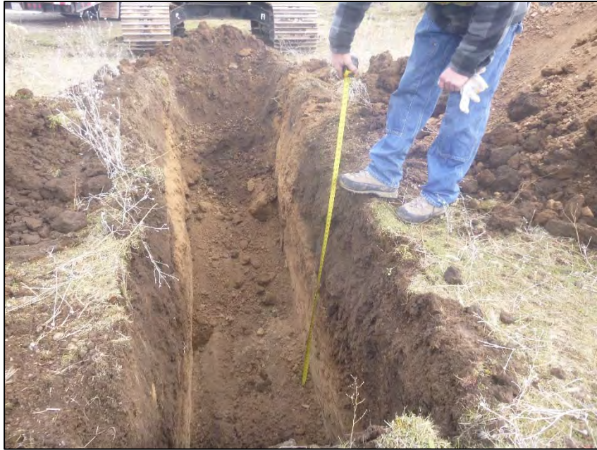
PHOTO 27 – TP-CO1-D pit excavated to depth 4.8 ft
