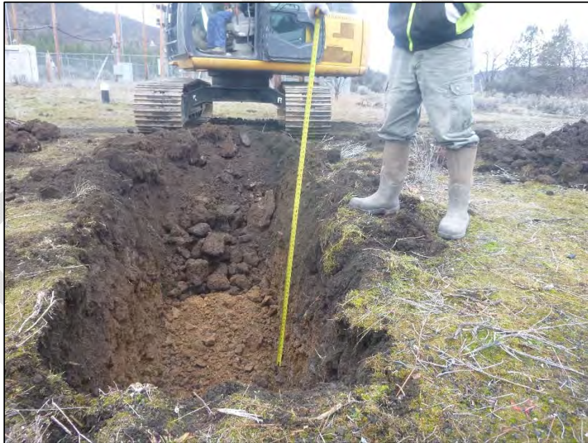
PHOTO 18 – TP-CO1-C pit excavated to depth 3.3 ft
