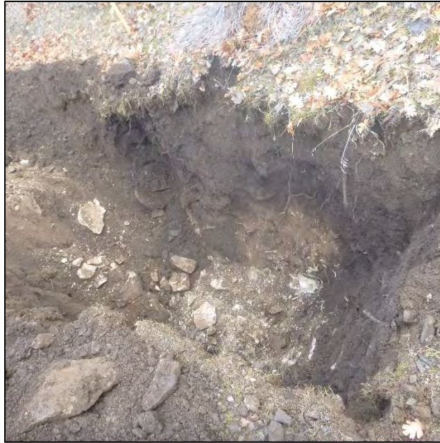
PHOTO 41 – TP-CO2-A pit excavated to final depth 5.8 ft
