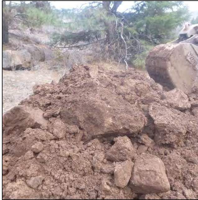
PHOTO 145 – TP-JCB-F spoils and boulders from depth 6.4 to 8.5 ft
