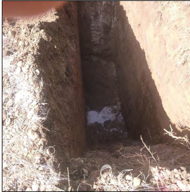
PHOTO 129 – TP-JCB-D pit excavated to depth 8.8 ft
