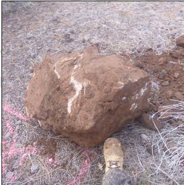
PHOTO 134 – TP-JCB-E boulder uncovered approximately 2.0 ft below surface
