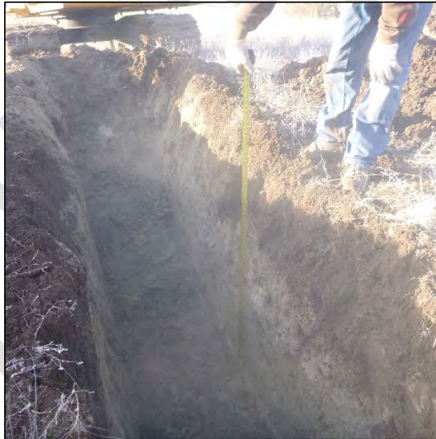
PHOTO 72 – TP-IG-C pit excavated to final depth 5.6 ft
