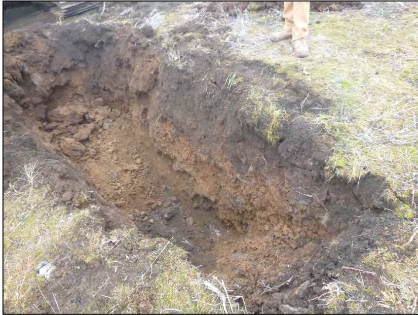
PHOTO 21 – TP-CO1-C pit excavated to final depth 5.5 ft
