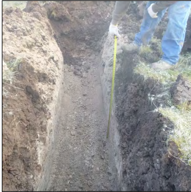
PHOTO 55 – TP-IG-A pit excavated to depth 4.6 ft
