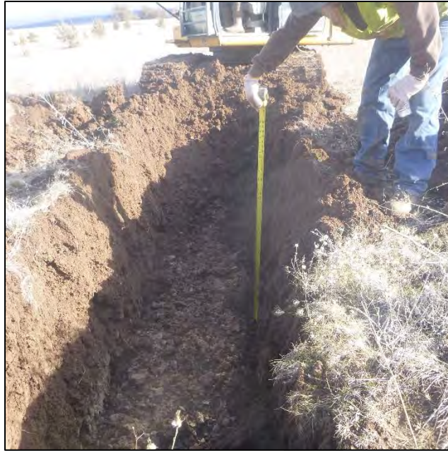
PHOTO 61 – TP-IG-B pit excavated to depth 3.0 ft
