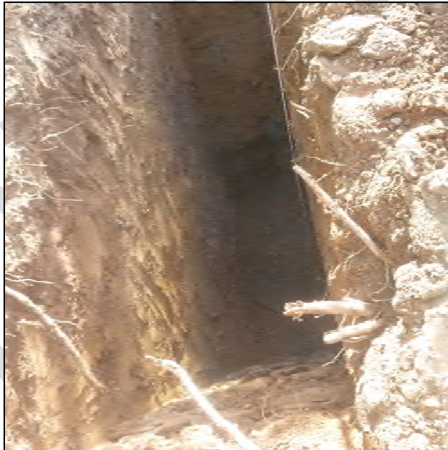
PHOTO 110 – TP-JCB-B pit excavated to depth 12.0 ft
