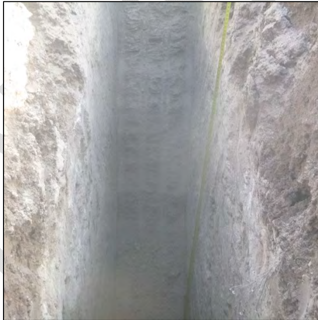
PHOTO 66 – TP-IG-B pit excavated to final depth 15.0 ft
